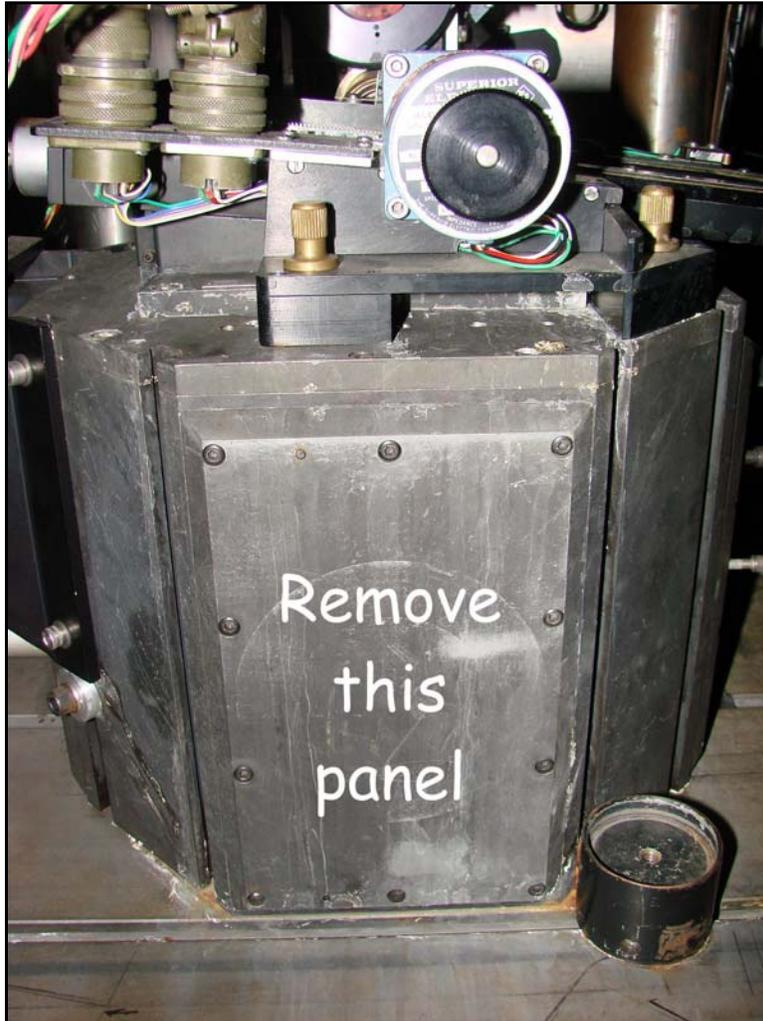
Remove the panel screws. The panel is pinned so some gentle prying will be needed.
